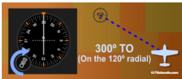
Rotate the Omni-Bearing Selector (OBS) until the needle centers. It is best to select the bearing to or from the station that corresponds to the direction inbound or outbound of the desired track.
