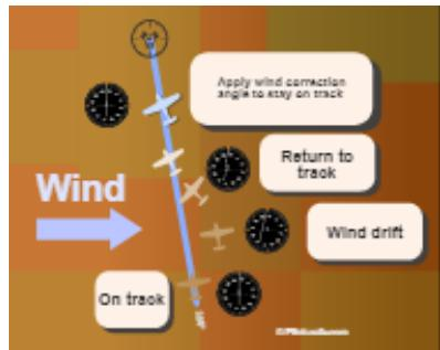
If you don't know the wind direction, you'll have to find the best correction by trial and error. Otherwise, an E6B, FMS or a electronic flight computer can calculate it for you.
