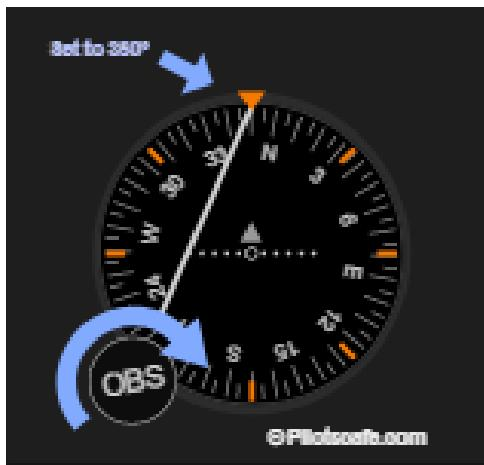
The bearing displayed on the top of the dial is your current bearing to or from the station.
