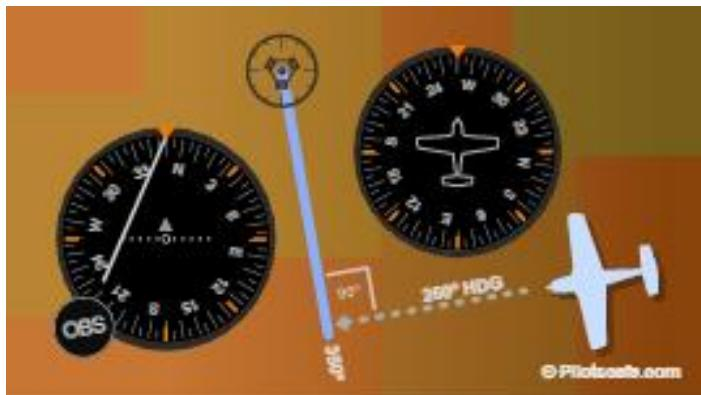
Note to which side the needle deflected (left or right.) To intercept the course, fly towards the needle with the intercept angle you chose in step 2.
