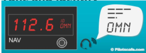
Before using a VOR for navigation, you must tune its frequency and make sure you are receiving the correct station.
