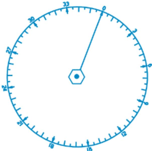
We could be on any one of these radials being emitted from the station. We can use our instrument in the cockpit to tune to a VOR and track TO the station or FROM the station on a selected radial.
